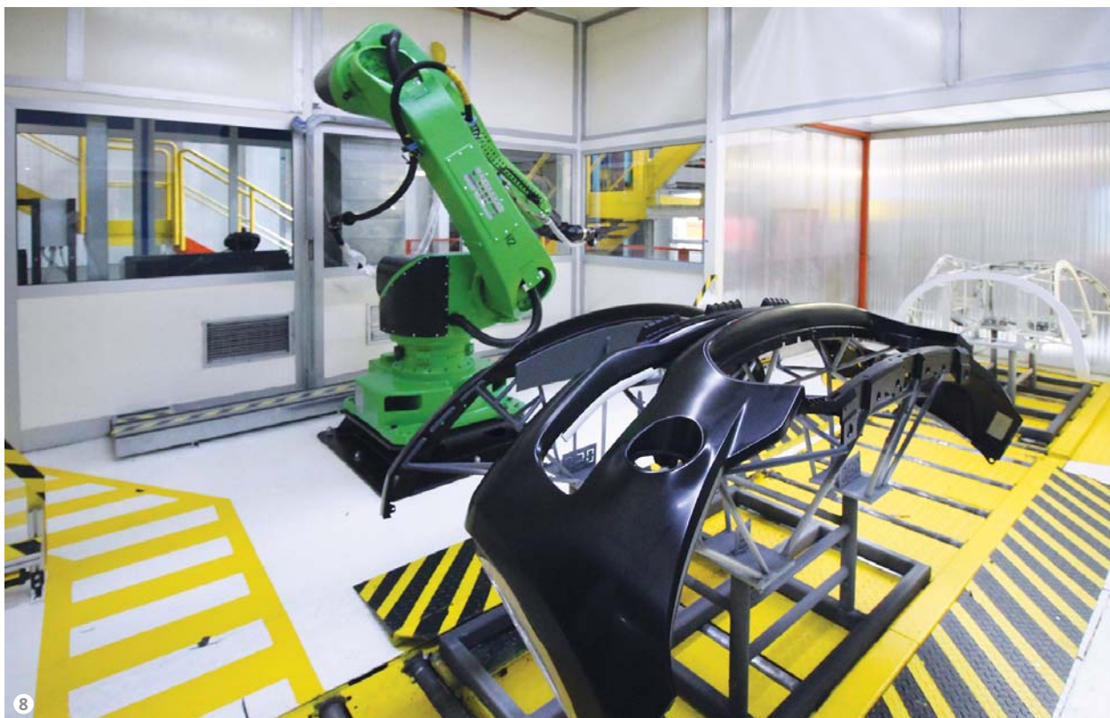
Figure 8: Each skid can house 1 to 4 components depending on the type and size of the workpieces: for instance, only one bumper and its strip or, alternatively, 4 smaller size mouldings can be arranged.
