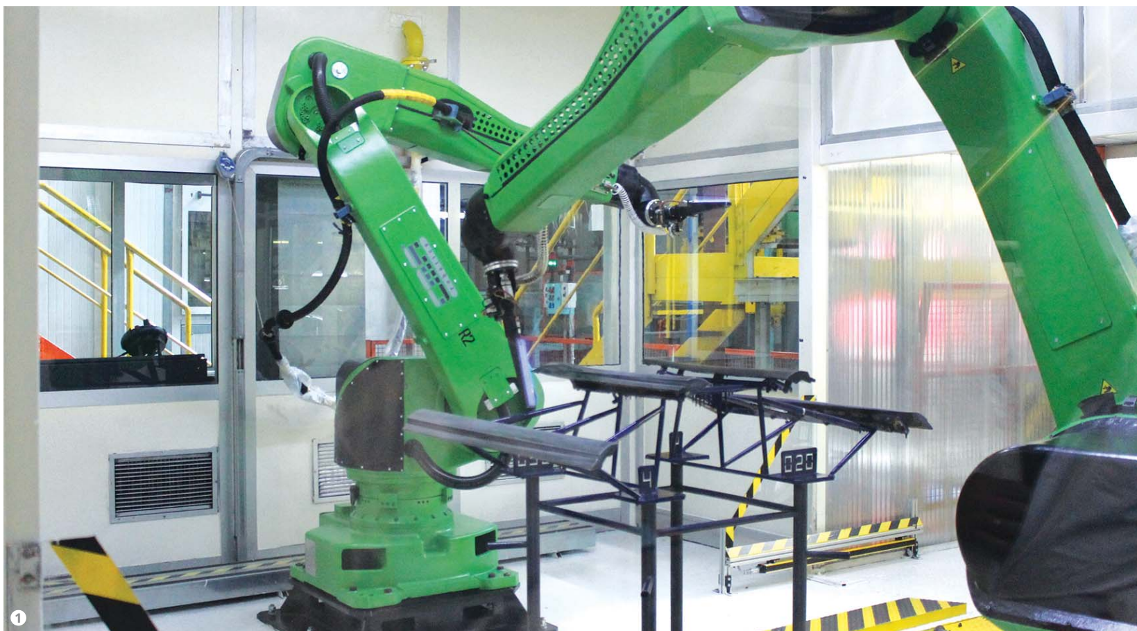
Figure 1: The two robots for flame hardening plastic bumpers built by CMA Robotics (Pradamano, Udine).
