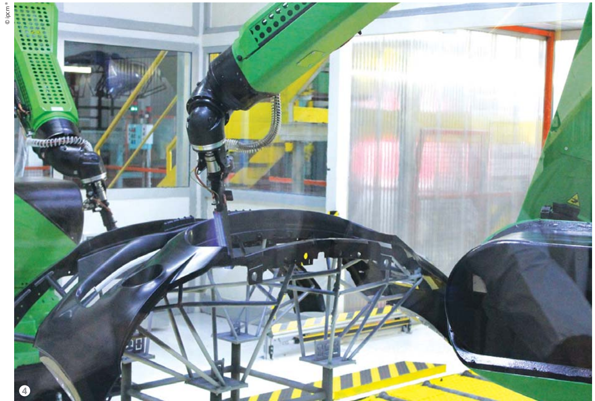
Figure 4: Bumpers subjected to flame hardening.
