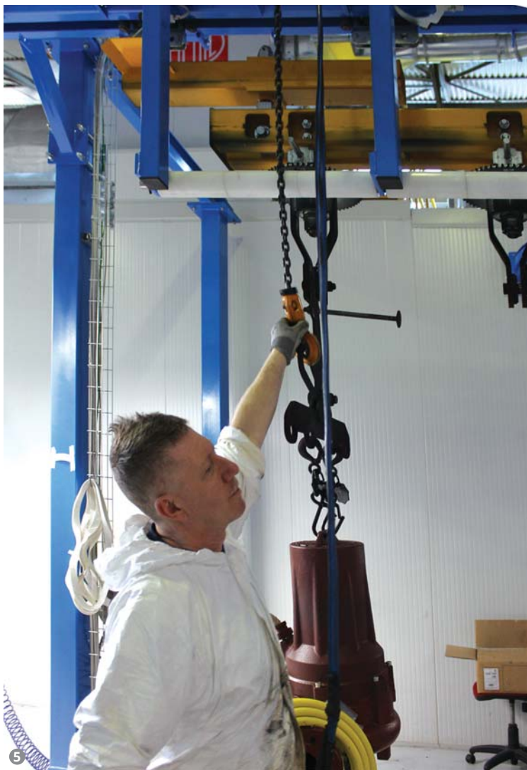
Figure 5: Each load bar has a maximum capacity of 1800 kg, up to 1000 kg per hook.
