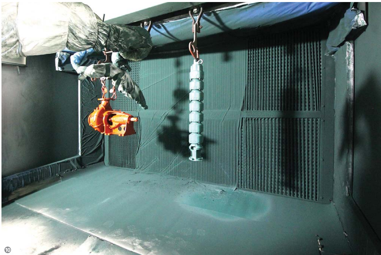
© ipcm ® Figure 10: The dry application booth devoted to enamel.
