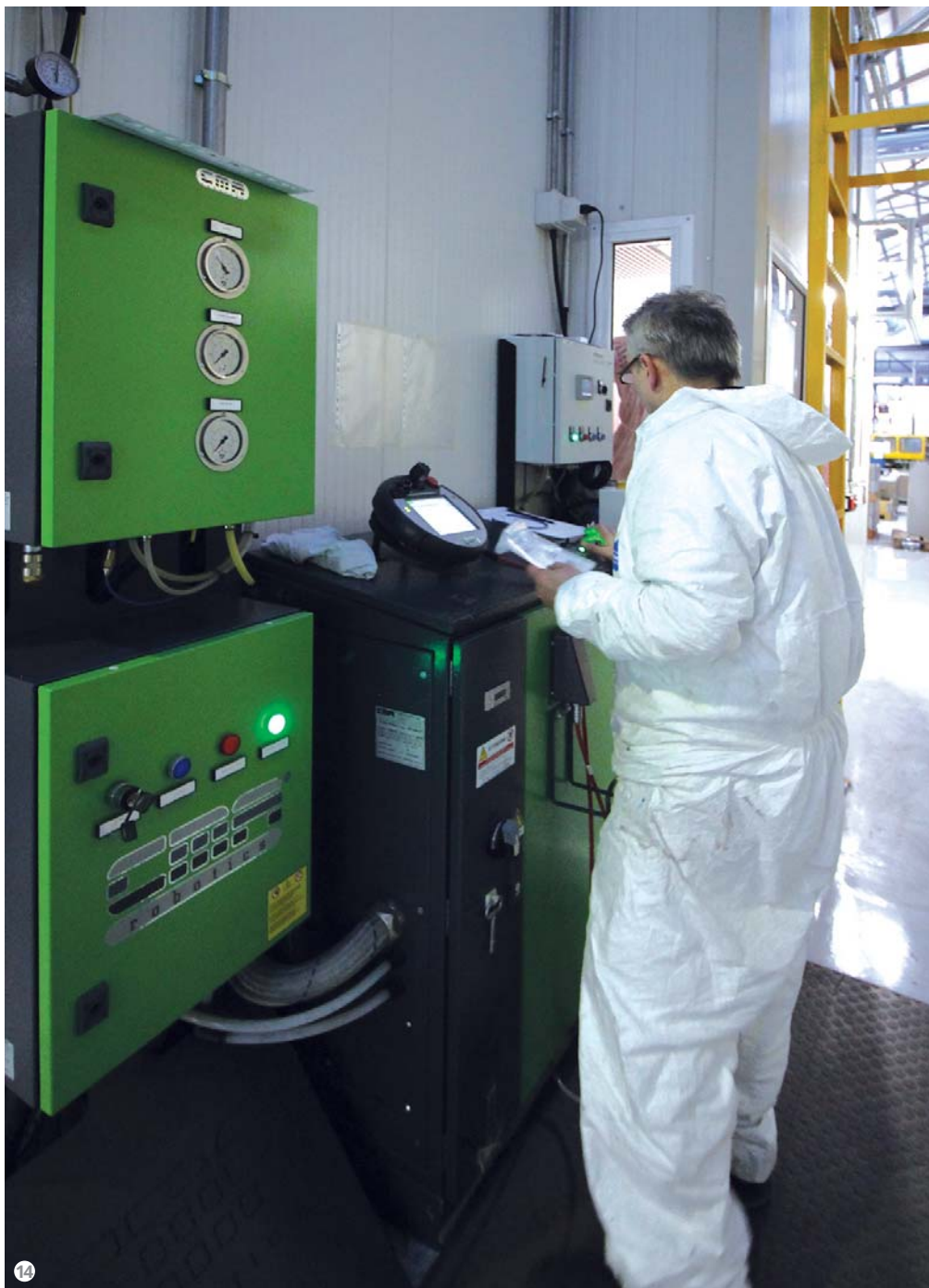
Figure 14: One of the stations for the management of the robots installed by CMA (Pradamano, Udine).
